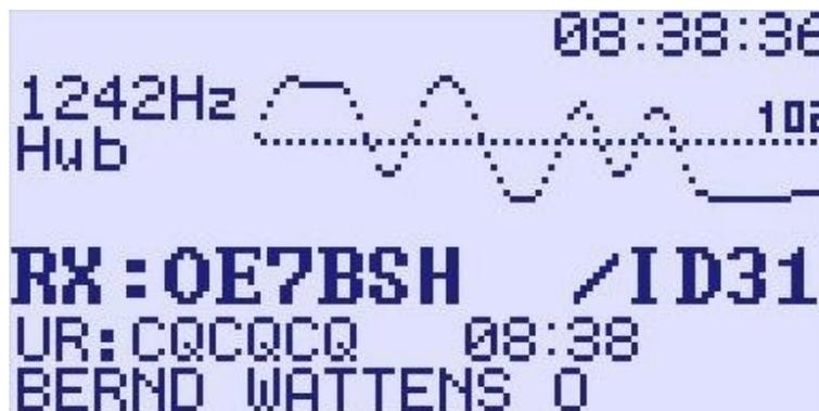
**Figure 27: Hotspot operation, displaying the hub of the received signal**
